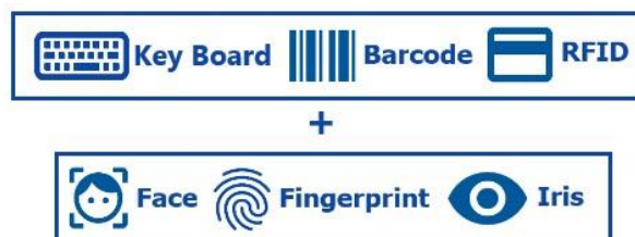
Figure 6.161 Combinations of user id peripheral with biometric peripheral in verification mode
