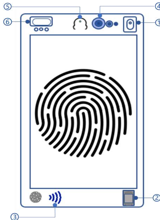
Figure 3.1 Picture with example device with fingerprint scanner, Temperature sensor and Motion Sensor functionality
